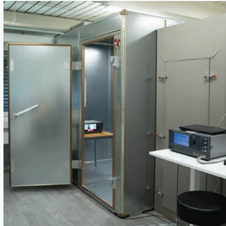
Ferronato's Faraday cage in our testing facility in Châtel-St-Denis, Switzerland.
